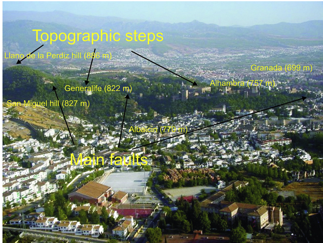
Fig. 3. Relationship between the following steps in the relief and faults: Llano de la Perdiz–Generalife, San Miguel hill–Albalcín, Generalife–Alhambra and Alhambra–Granada.
