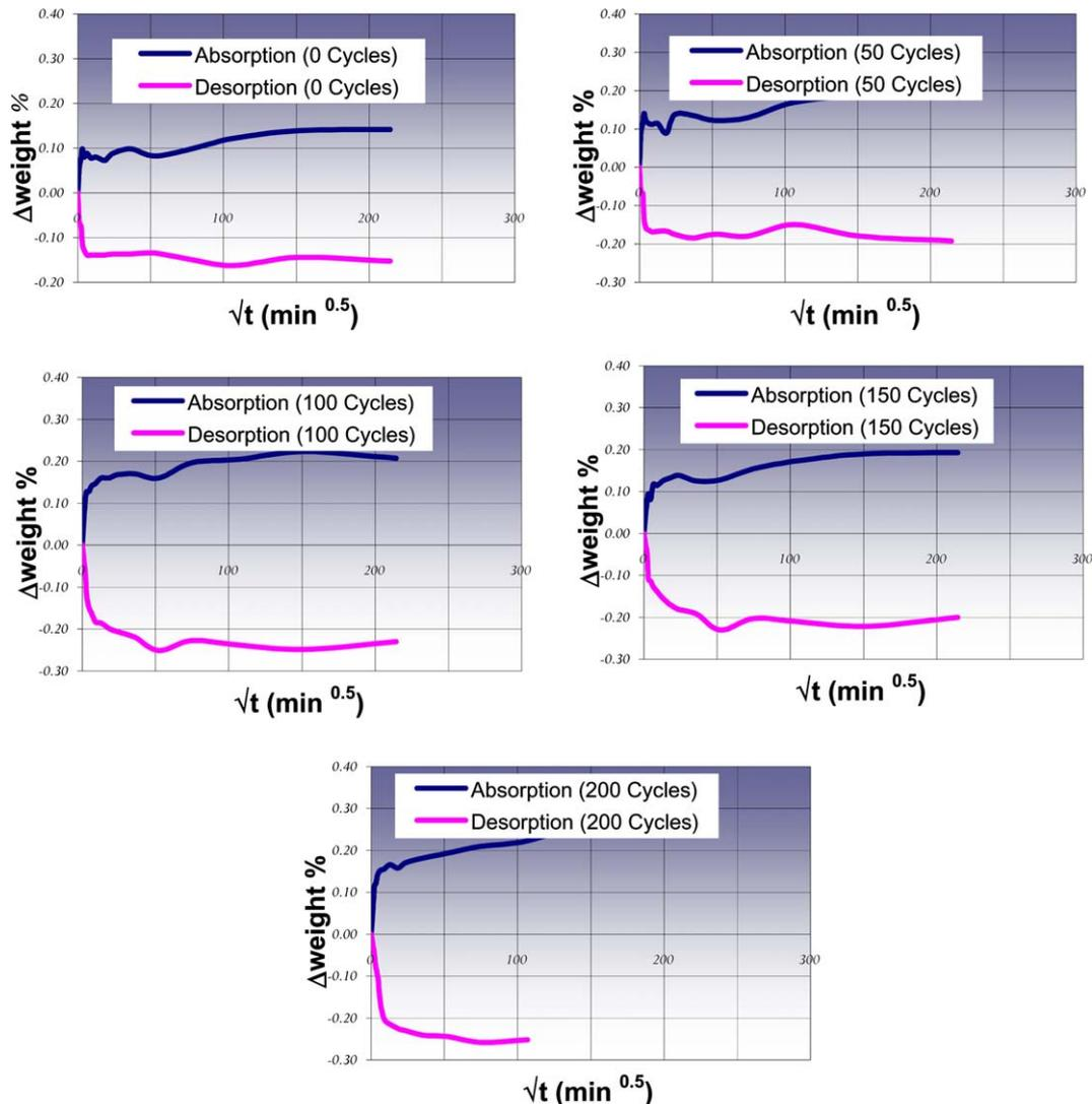
Fig. 7. Absorption and desorption curves for material from groups A and C after the series of cycles established.
