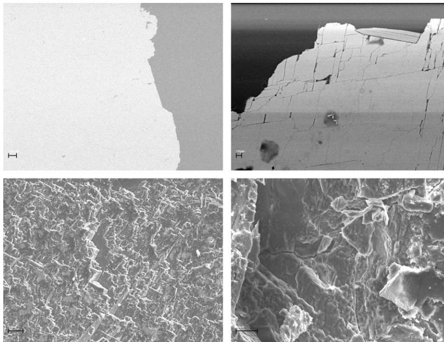
Fig. 8. (Upper left) SEM image of thin section from block (0 cycles) – considerable homogeneity can be observed. (Upper right) SEM image of thin section from block (200 cycles) – rhombohedral exfoliation of calcite crystals is especially noticeable in the external zone. (Lower left) – SEM image of fragment from block (0 cycles) – the homogeneous nature of the sample is noticeable. (Lower right) SEM image of fragment from block (200 cycles) – microfracturing and disaggregation are noticeable.
