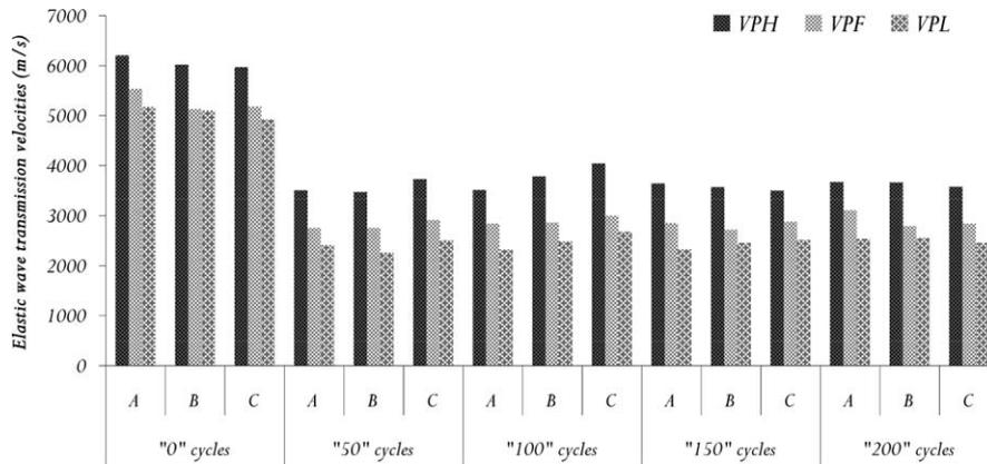
Fig. 5. Variability of elastic wave transmission velocities in the material for each of the groups (A, B and C) according to the three directions analysed (PV<sub>H</sub>, PV<sub>F</sub> and PV<sub>L</sub>) for each series of cycles (0, 50, 100, 150 and 200).
