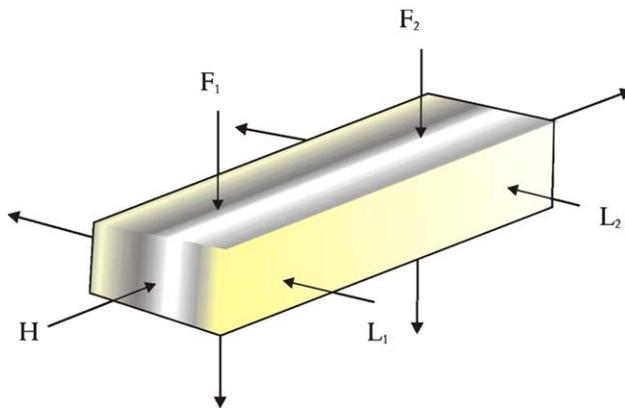
Fig. 3. Diagram of ultrasonic propagation velocity directions measured in each block.
