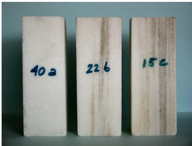
Fig. 2. Detail of the groups of sample blocks established: (a) (absence of banding), (b) (intermediate banding) and (c) (abundant banding).
