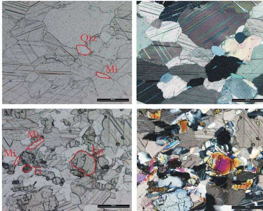
Fig. 4. (Upper part) Detailed view of accessory minerals (quartz and mica). Note the coinciding lengthening of the colourless mica and calcite crystals. (Left) one polariser, (right) crossed polarisers. (Lower part) General view of the concentration of accessory minerals (mainly epidote and titanite) in dark levels of the grey sample. (Left) one polariser, (right) crossed polarisers.
