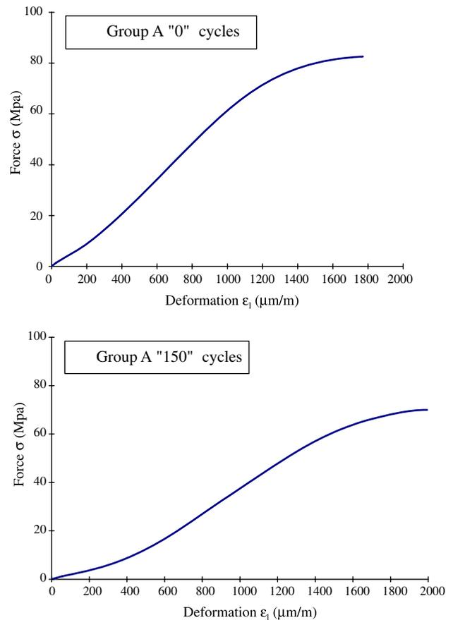
Fig. 6. Force–deformation curves for Group A blocks not subjected to cycles and after 150 cycles.
